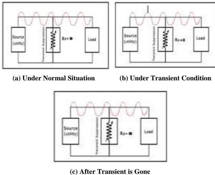
Figure 1: Metal Oxide Varistor (MOV) Current Divider
