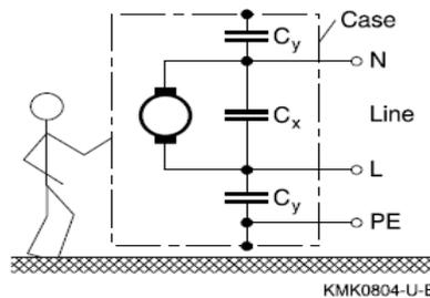
**Figure 4: Application of X & Y Capacitor**
